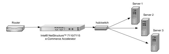
Figure 3-2: 7110/7115 in Multiple Server Configuration
